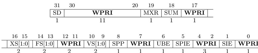
Figure 8.21: Virtual supervisor status register (`vsstatus`) when VSXLEN=32.
