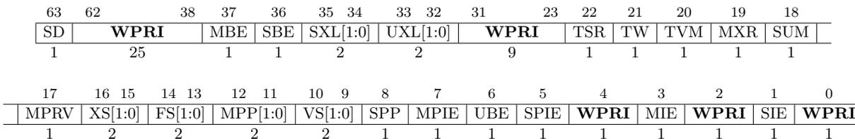
Figure 3.7: Machine-mode status register (`mstatus`) for RV64.
